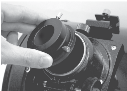
Figure 22a. First remove both the 1.25" and 2" adapters as shown
