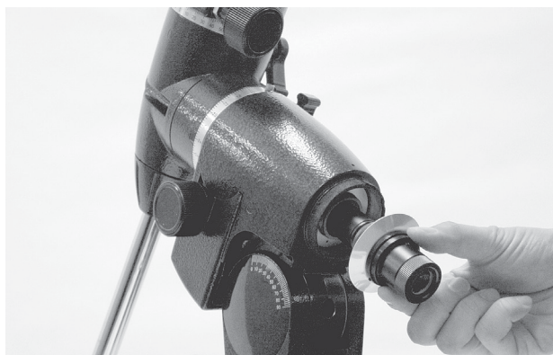
Figure 10b. Installing the optional polar axis finder scope.
