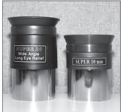
Figure 9: The 20mm and 10mm eyepieces
