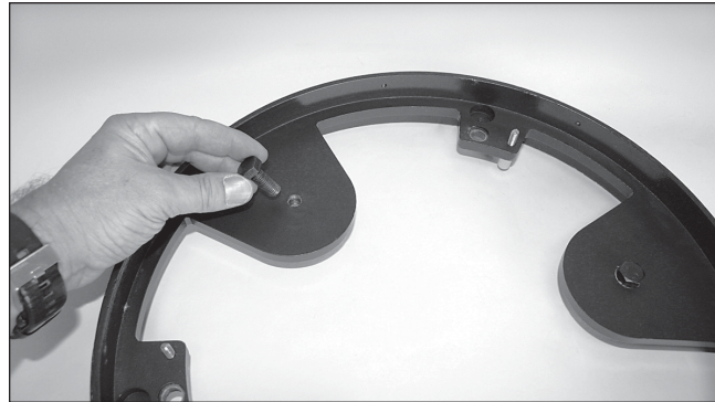
Figure 15. Thread the three hex-head counterweight mounting bolts (XX14g and XX16g only) into the holes in the counterweight support plates as shown. Tighten using an adjustable or 16mm crescent wrench.
