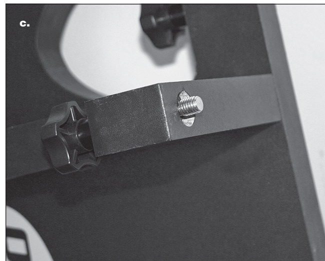
Figure 9. a) Place a rubber washer on the threaded end of the connecting bolt and push it on as far as you can with your fingers. b) Then use the included insertion tube to push the washer past the threads and up into the counterbored hole in the wood. c) The recessed washer will keep the bolt captive in the hole.
