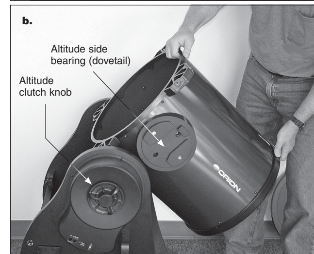
Figure 18. a) Altitude axis trunnion on left side panel. b) Grasp both ends of the lower tube section to lift it, then lower it into the base, sliding the dovetail slot in the tube's left altitude bearing into the mating part of the trunnion.
