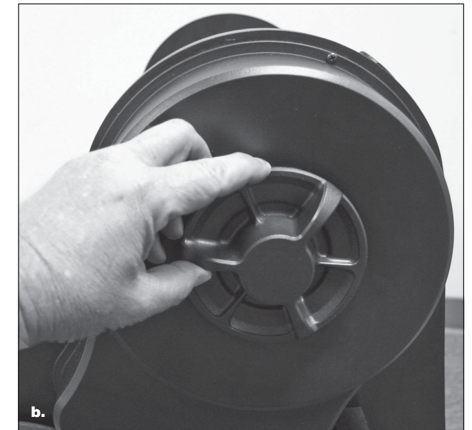
Figure 34. a) The redesigned altitude (Alt) and (AZ) azimuth motor/encoder housings of the XXg Dobs feature large manual clutch knobs for adjustable motion tension. b) Rotate the clutch knob to adjust the friction of motion for slewing the telescope by hand.
