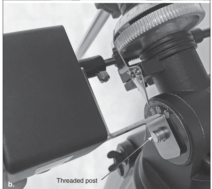
Figure 7. a) First fasten the drive coupler onto the R.A. gear shaft, aligning the thumbscrew with the groove on the shaft end. b) Then place the bracket hole over the threaded post.
