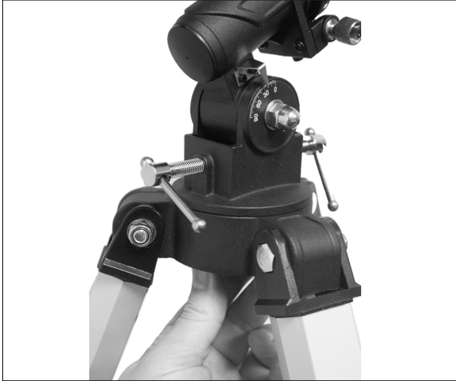
Figure 2. Attach the EQ head to the tripod by threaded the large thumb knob up from below until the EQ head is snug against the tripod.
